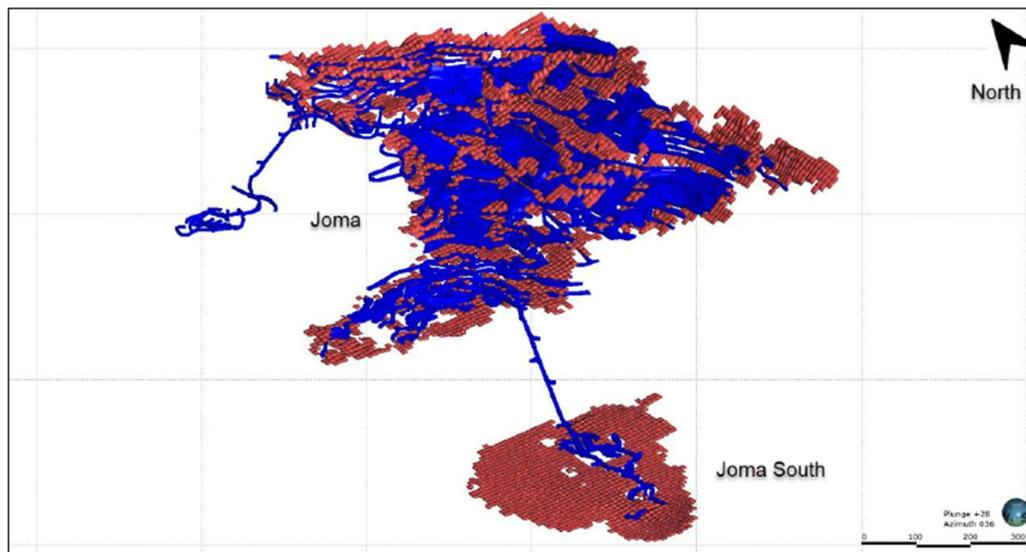
**Figure 10: North-east view of the MSO shapes (red) in relation to the depletion survey (blue). The MSO shapes have been used to constrain the reporting of the Mineral Resources**
