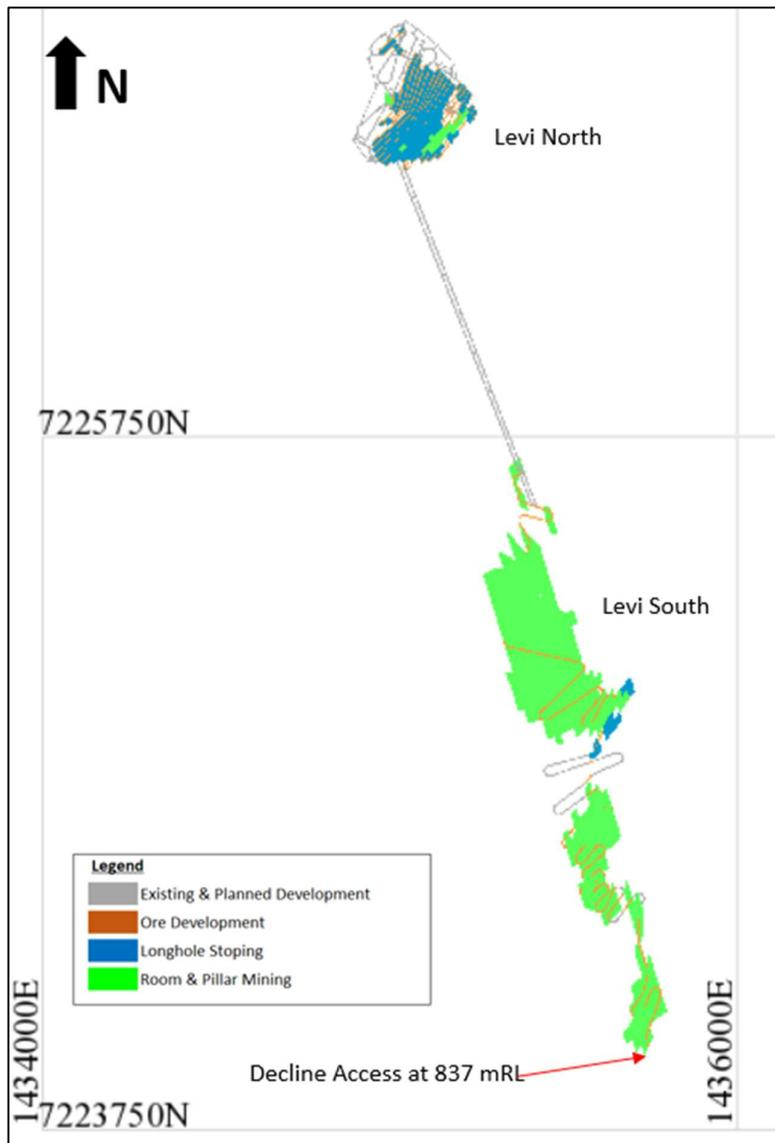
**Figure 16: Plan view of the Levi Mining Inventory by mining method and existing and planned development**
