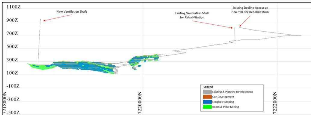
**Figure 15: Long view of the Stekenjokk Mining Inventory by mining method and existing and planned development, looking northwest**
