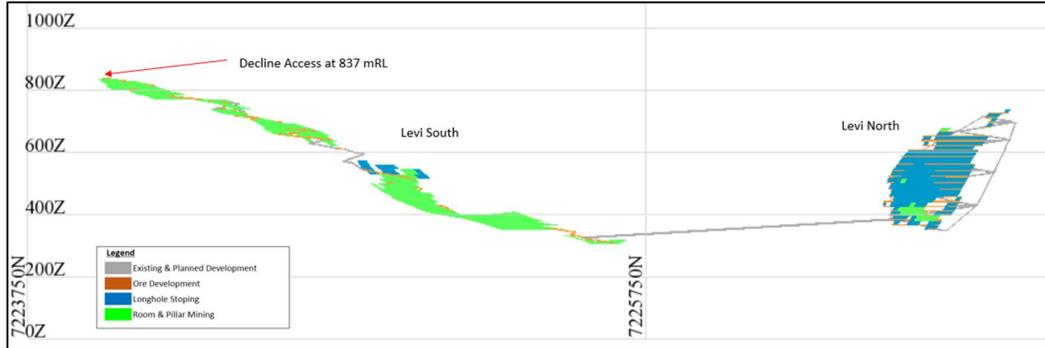
**Figure 17: Long view of the Levi Mining Inventory by mining method and existing and planned development, looking southwest**
