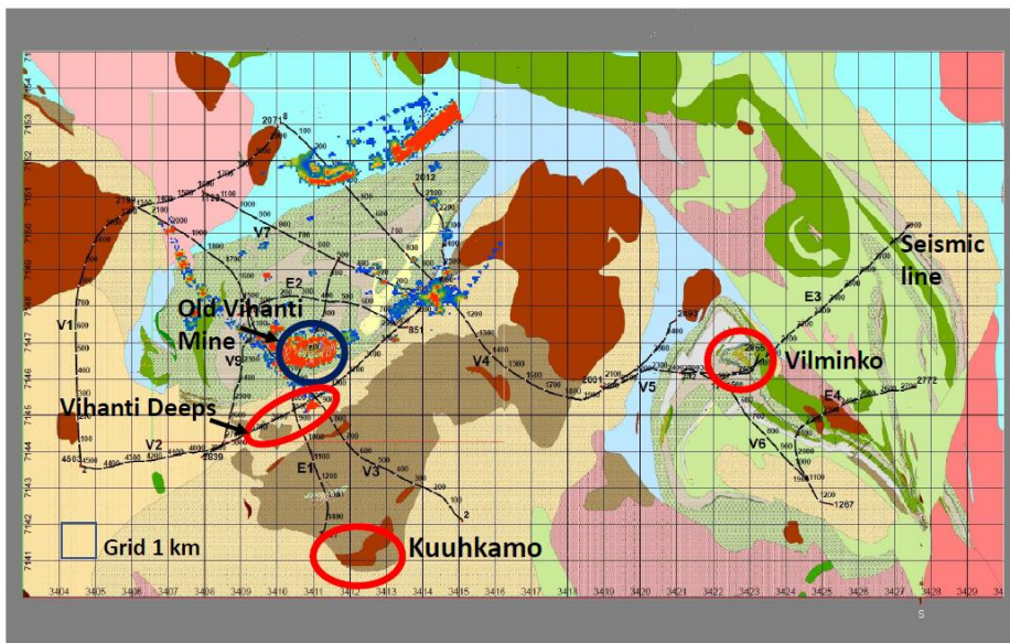
Fig. 3. Three drill targets: Vihanti Deeps, Vilminko and Kuuhkamo on a geological map also showing the closed Vihanti mine and lines in a seismic survey.
